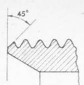
CHAMFER TO ROOT OF THREADS
