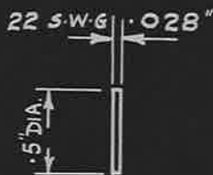
FLAT DISC PART 3 MATERIAL - BRASS, HARD ROLLED SPEC. B 5 SCALE - 1/1.
