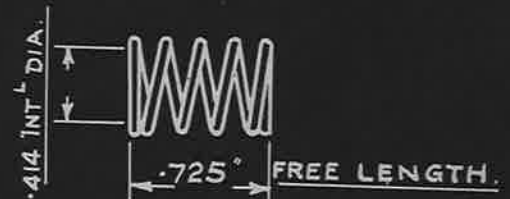
SPRING PART 4 MATERIAL - HARD DRAWN STEEL WIRE SPEC. D.T.D. 5A SCALE - 1/1
