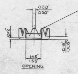
SPACED, COMMENCING EACH SIDE OF OPENING WITH HALF SERRATION
