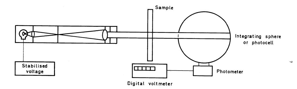
Fig 1 Measurement of in-line visual light transmission
