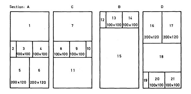
Fig 1 Standard cutting plan for test specimens
