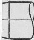
The ends to be shaped to fit the Axial loading shackles of the testing machine
