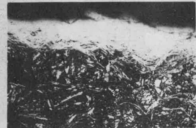
Sun Gear 500X Nitrided Case and white layer; 974 VDH 2% Nital etch
