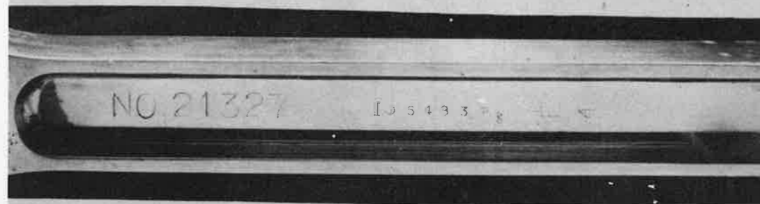
Figure 4 . Articulated Rod Showing Numbers Stamped in the Polished Surface (CEE-2963). 30979
