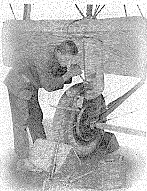
Plate 6.—Checking the Air Pressure after having blown off the excess oil.
